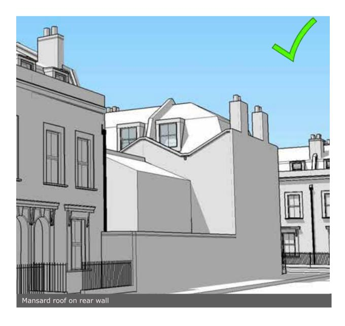
Rear view with mansard profiled gable - Outboard staircase
