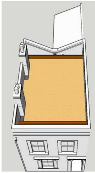
Install a roof framework which may include steel beams to support the mansard roof. The designer should consider how they will be lifted into place and installed
