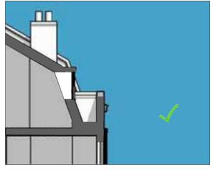
Double dormers would be subordinate when set back sufficiently and constructued with a narrow profile
