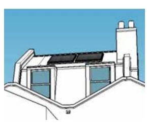
In-line panels sit flush with the roof and look more like rooflights
