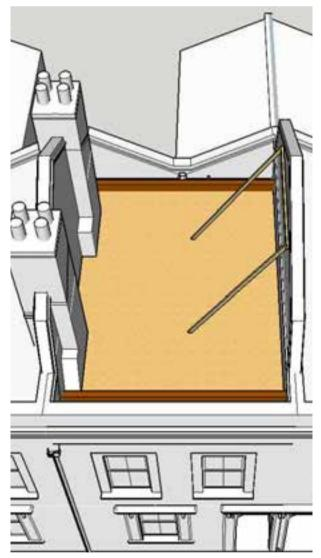
Raise the level of the party wall once temporary props are in place to restrain the party wall until the roof joists are tied in; the designer should consider all stages of work
