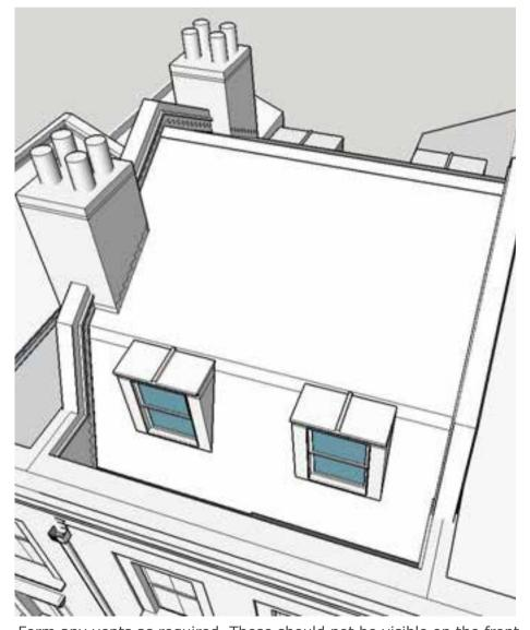
Form any vents as required. These should not be visible on the front slope. Fix slate to pitched roofs with lead lining to gutters, dormers and flashings
