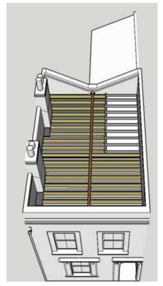
Fix new floor joists between ceiling joists supported on the bressemer beam and party walls. A structural engineer will need to design the roof framework to distribute the loads to the existing foundations
