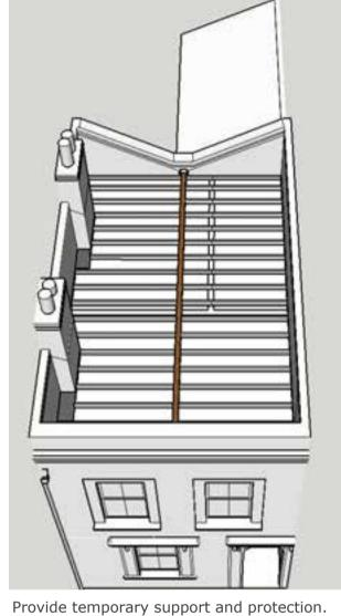
Provide temporary support and protection. Demolish the existing London roof. A structural engineer should inspect all structural elements. Repair and strengthen as required
